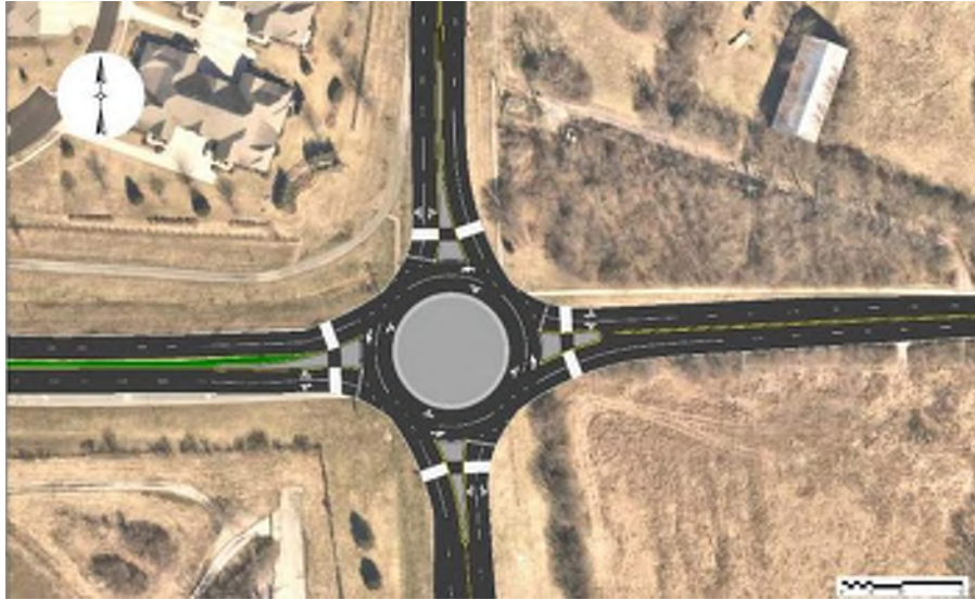
Figure 2: Dual Lane Roundabout
